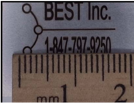
Figure 5 Laser markings on stainless steel
