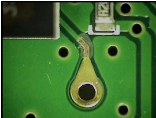
Figure 4 Laser etching of solder mask to extend a trace
